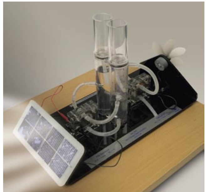
Sollys → el → brint+ilt → el+vand → ventilator drejer rundt
